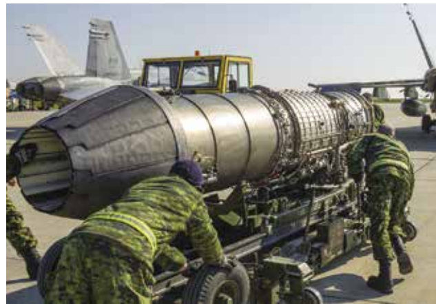
Technicians from Air Task Force-Romania change one engine on a CF-188 Hornet in Constanta, Romania during Exercise RESILIENT RESOLVE on March 17, 2016
